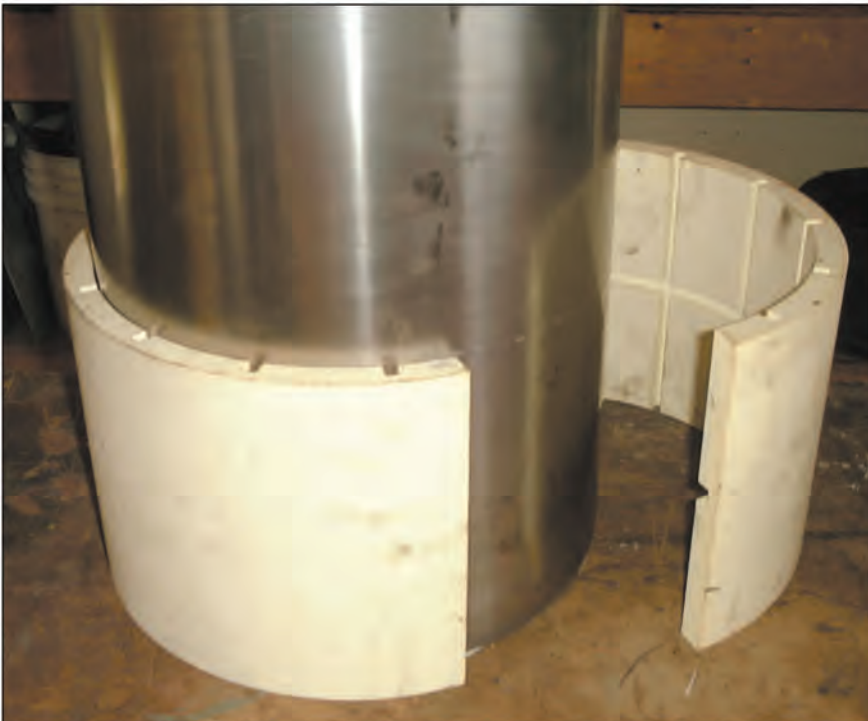
Photo 3. Fitting to the shaft
