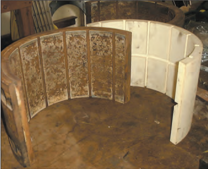
Photo 2. Bronze and elastomer, side by side
