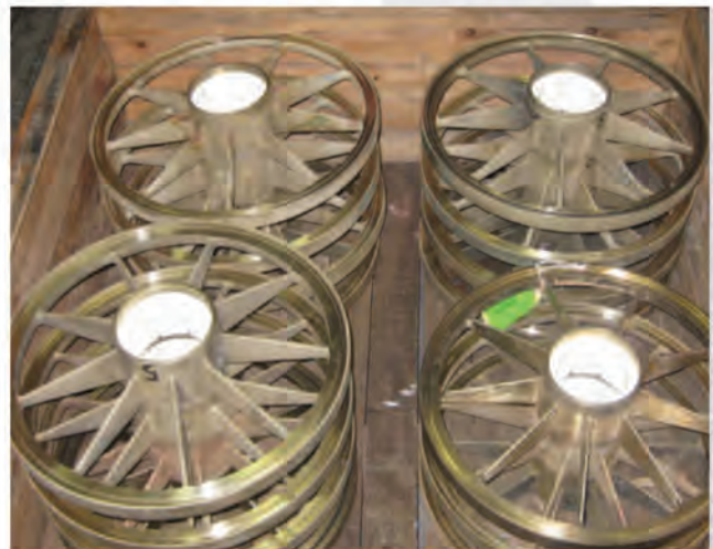
Thordon SXL pump bearings installed into existing bronze
